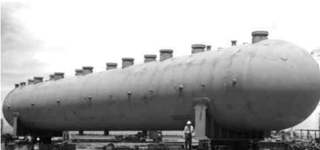
Figure 1: Titanium clad steel PAL autoclave at the Murin Murin Nickel Cobalt Project. (photograph provided by ASC Engineering)
