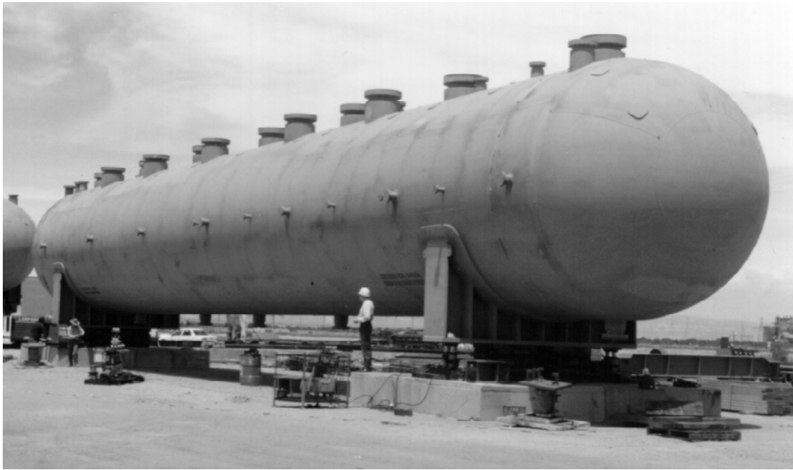
Figure 1: Titanium clad autoclave for nickel laterite pressure acid leaching. The autoclave is Titanium Grade 1 clad steel for the Murin Murin Nickel / Cobalt Project. Photo provided by the autoclave fabricator, ASC Engineering, Adelaide, Australia.
