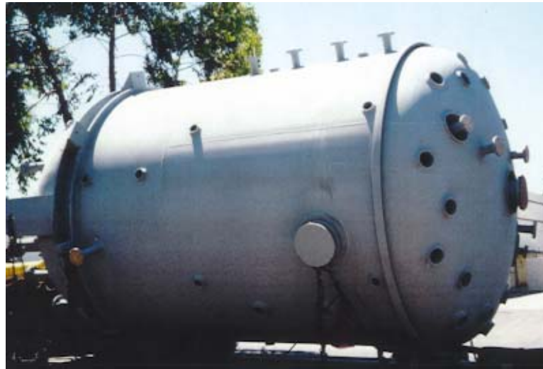
Figure 3: A typical jacketed zirconium-steel clad pressure vessel.
