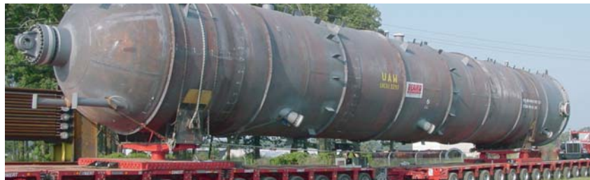
Stainless steel clad refinery column. 180 inch ID x 116 feet long x (4 inch Cr-Mo steel + 0.12 inch type 321 stainless steel.)
