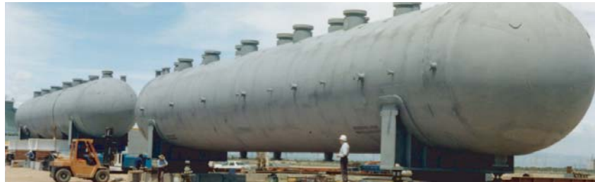
Titanium-Steel clad autoclave for pressure acid leaching of nickel and cobalt ore. 204 inch ID x 115 feet long x (4 inch steel + 0.25 inch titanium)
