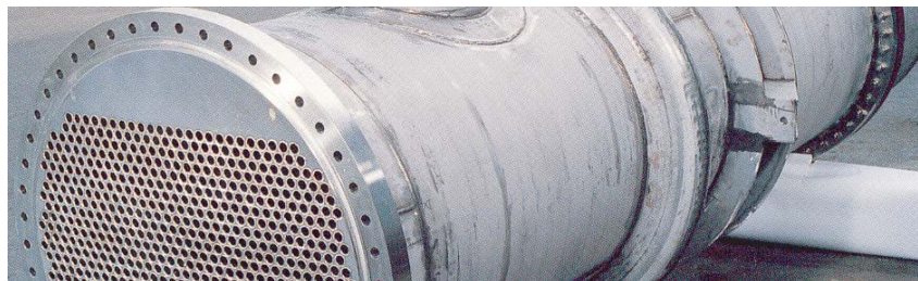
Nitric acid cooler condenser with zirconium tubes and 48 inch diameter zirconium + stainless steel clad tubesheet.
